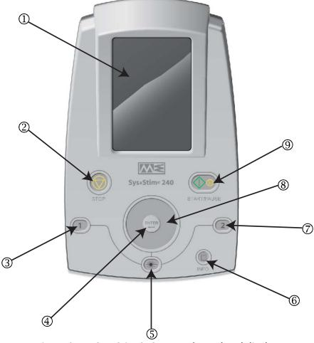
Figure 2.1— Sys\*Stim 240, control panel and display
