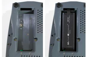
Figure 3.2— Sys\*Stim 240, Bottom View— Installing the battery
