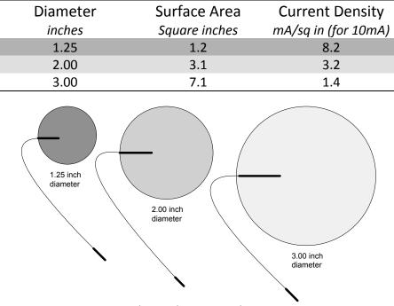
Figure 4.2—Electrode Sizes and Current Density
